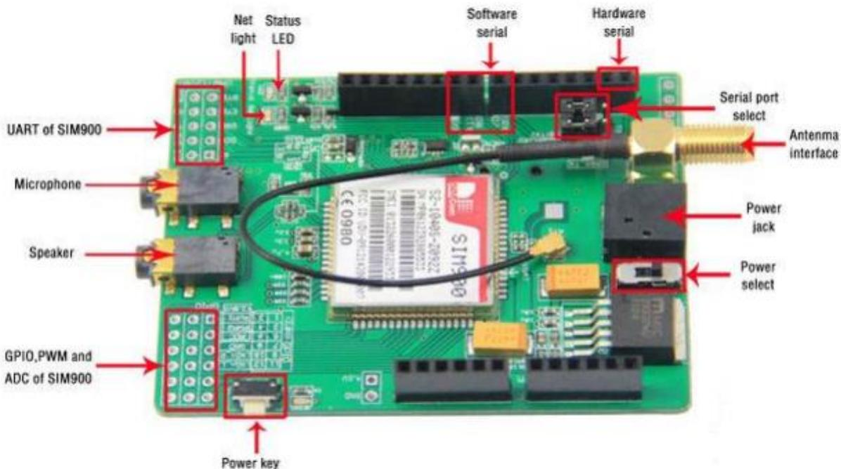
**Figure 4 A SIM900 GSM shield.**
